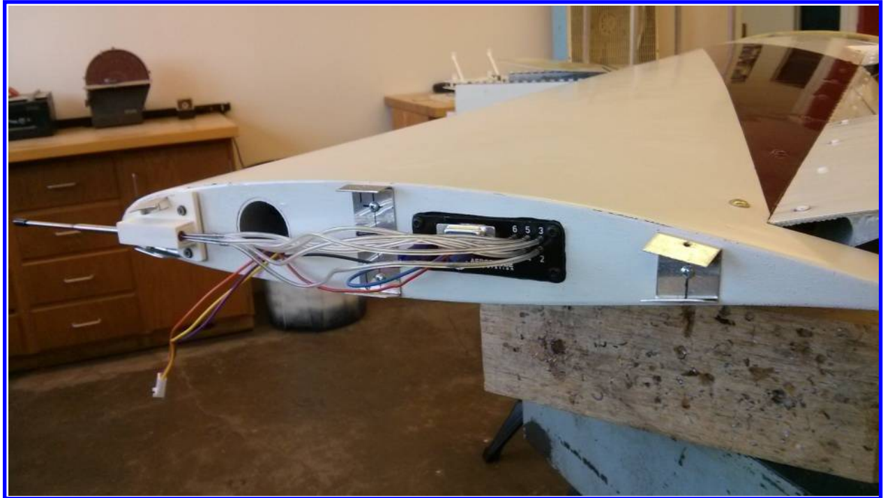
Figure 2. Internal installation of 5-hole air data probe and air data computer
