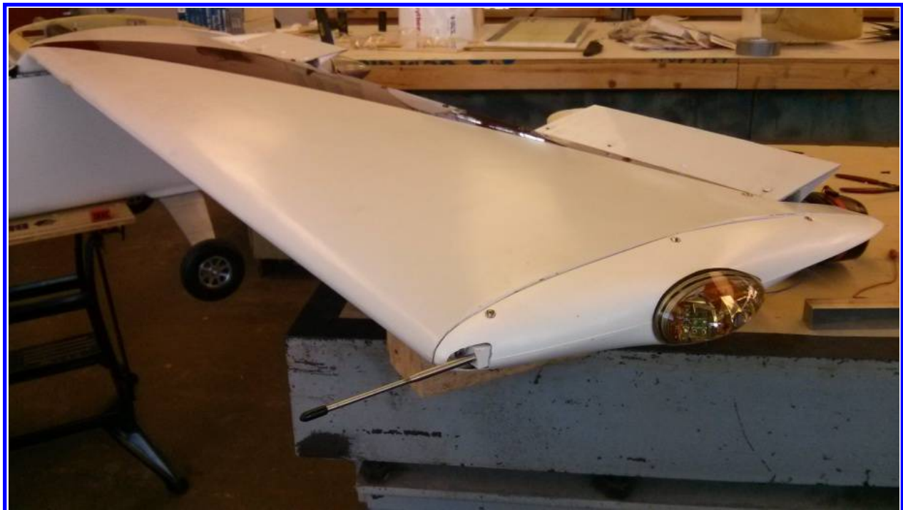
Figure 3. Wingtip installation of 5-hole air data probe
