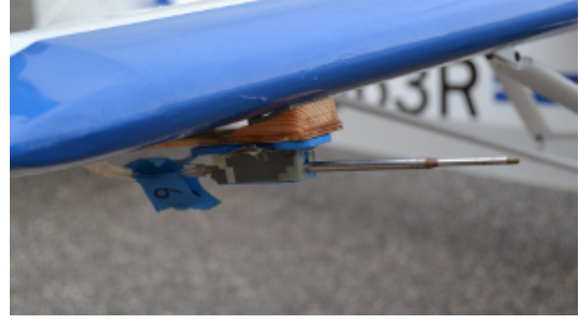
Fig. 4: Detail view of 5-Hole Probe mount.
