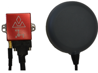
Fig. 5: VectorNav VN-200 Inertial Navigation System.
