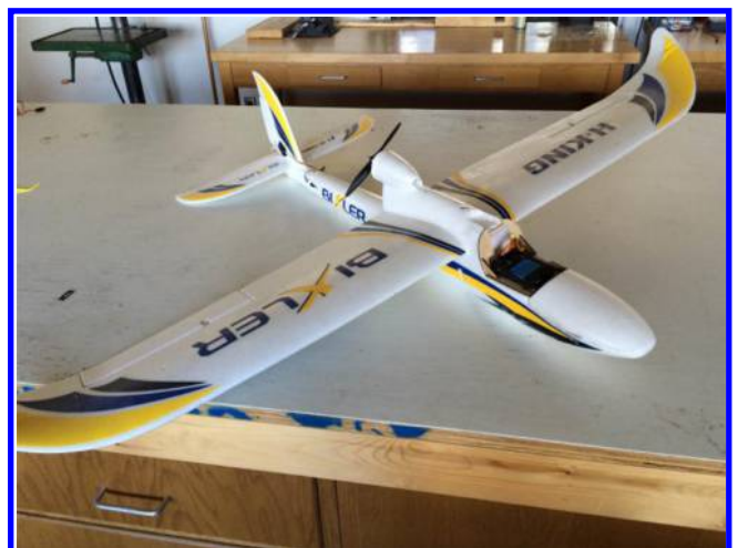
Fig. 1 Hobby King Bixler flight vehicle modified for autonomous flight testing. The Bixler has the same configuration and nearly identical dimensions to the Multiplex Easy Star.
