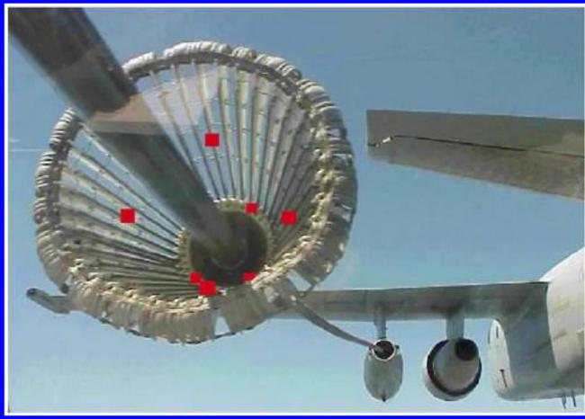
Fig. 2 Candidate beacon configuration for AAR, as seen from VisNav sensor.
